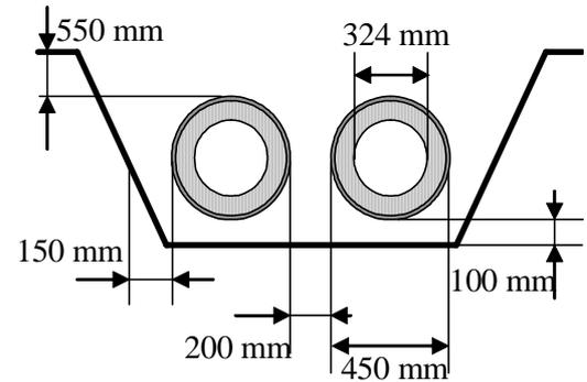
Figure 2. Schematic of the excavation.
