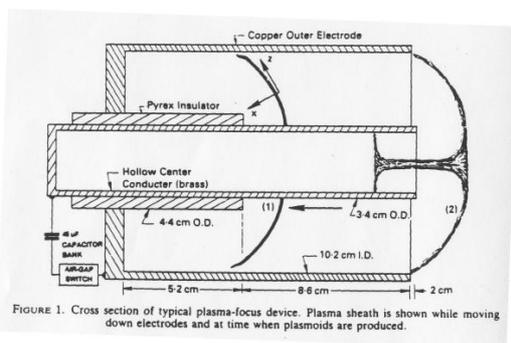
The chamber is filled with a dilute gas, decaborane, fed from the fuel chamber. (A kilogram of fuel will be sufficient for a year's operation.) The plasma focus consists of two copper electrodes nested inside each other with the outer one consisting of a circular array of rods and the inner one a single hollow copper rod.
